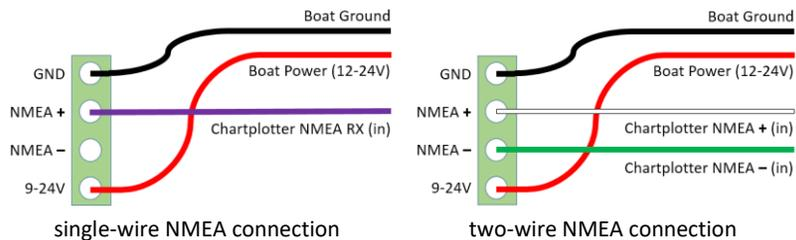
By default, dAISy 2+ is configured to output at 38400 Baud (NMEA high speed). This can be changed to other baud rates in the configuration and debug menu. You also need to check the configuration of your chartplotter. In many models, the NMEA port needs to be enabled in the settings menu and set to the correct protocol, like for example NMEA high speed).
