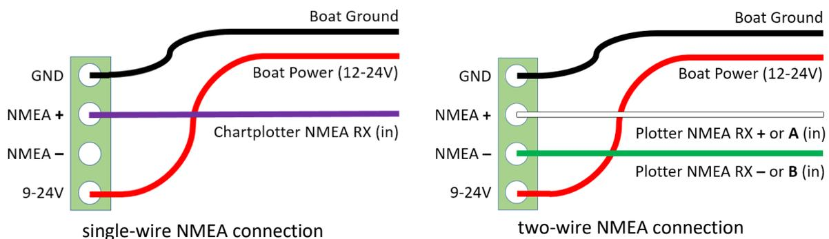
By default, dAISy is configured to output at 38400 Baud (NMEA high speed). This can be changed to other baud rates in the configuration and debug menu. You also need to check the configuration of your chartplotter. In many models, the NMEA port needs to be enabled in the settings menu and set to the correct protocol, like for example NMEA high speed).
